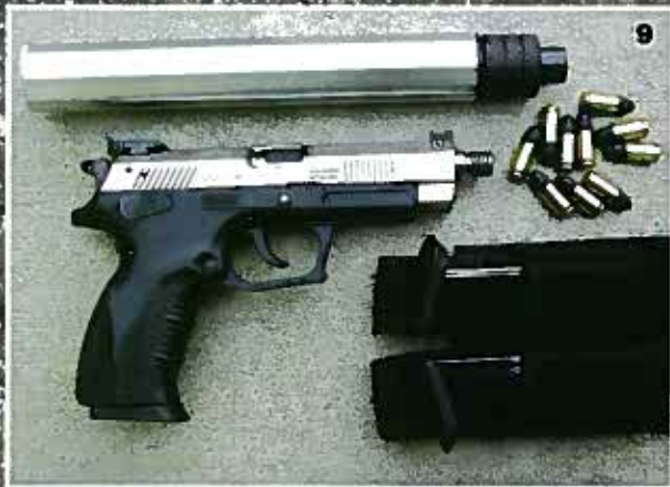
9: The K100 Whisper has a longer threaded barrel that enables the sound suppressor to be attached to it
